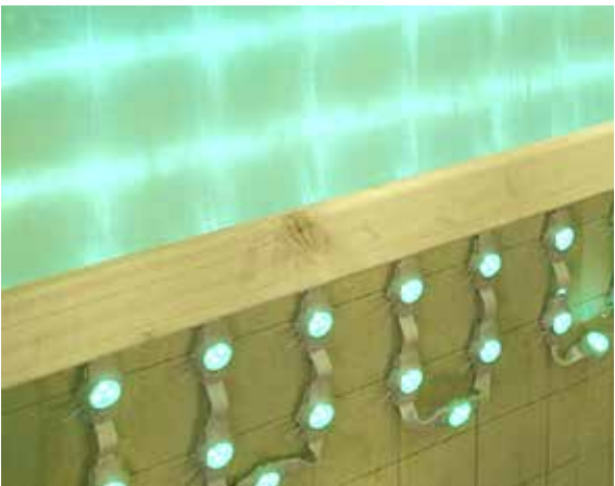
RESOLUTION TEST: PHYSICAL 1:1 MOCK-UP OF LED PIXELS
