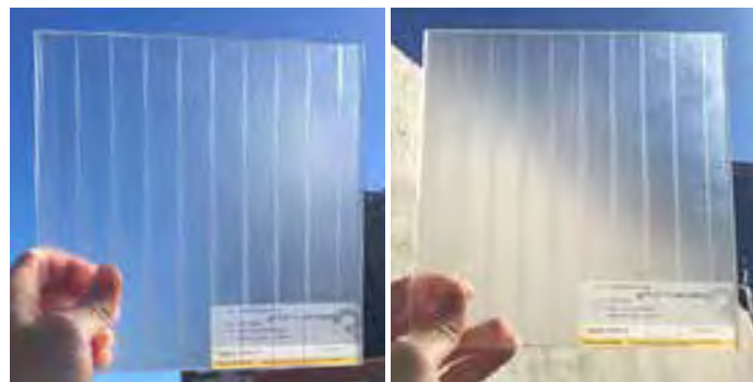
KODA XT, VELLUM FINISH WITH CUSTOM BACK TEXTURE STEP 3: CALIBRATING TEXTURE TO DESIRED OPACITY
