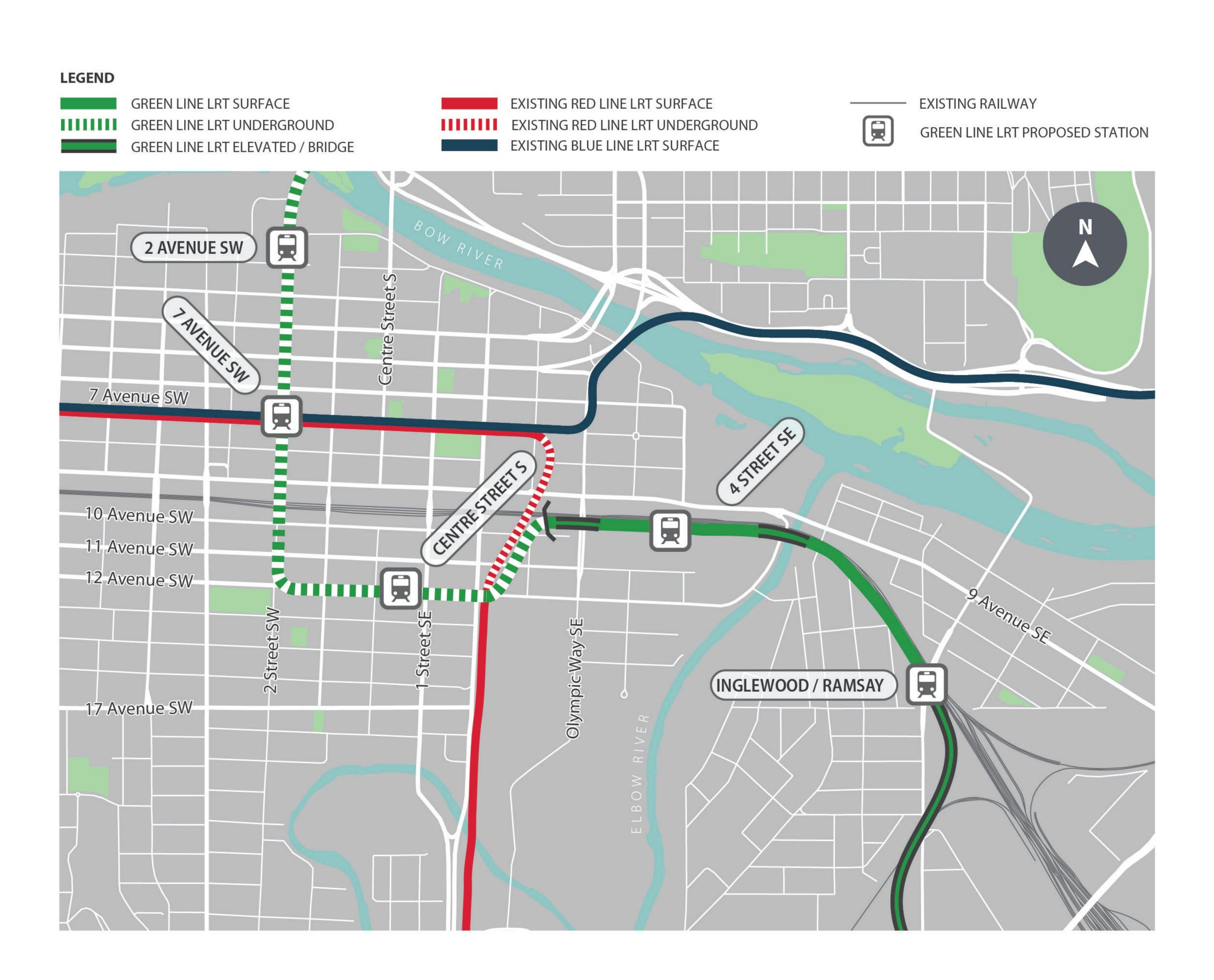
Would see the line jog north underground from the Centre Street station on 12 Avenue S to 10 Avenue S, where it would come to surface and run parallel to the south side of the CP tracks. This would:
